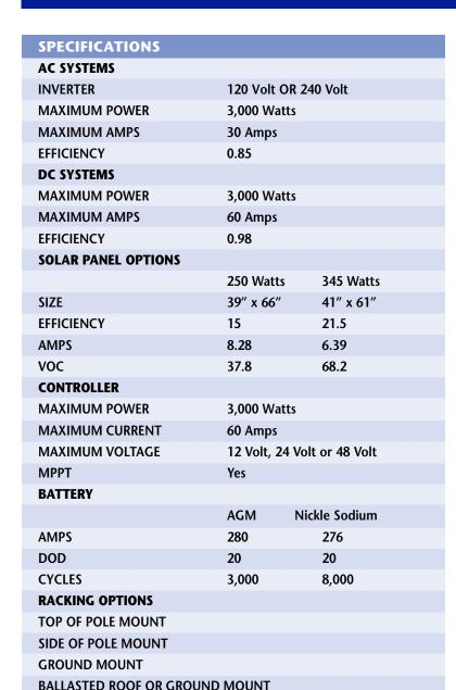
Because Solar installations are very site-specific, the options shown above can be modified and upgraded to deal with any project challenges. Sun-In-One<sup>™</sup> has over 10 years of experience and expertise in off-grid solar solutions. We design and manufacture power units that are interchangeable to maximize power for any location or conditions.
